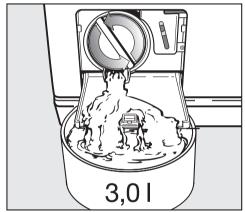
■ Turn the lint trap lid counterclockwise. **Do not remove it.** About 2 quarts of water will drain out of the hose.
